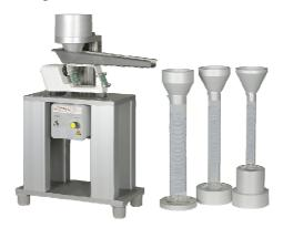
Tester for determination of the apparent density of granular activated carbon in accordance with ASTM D2854.
